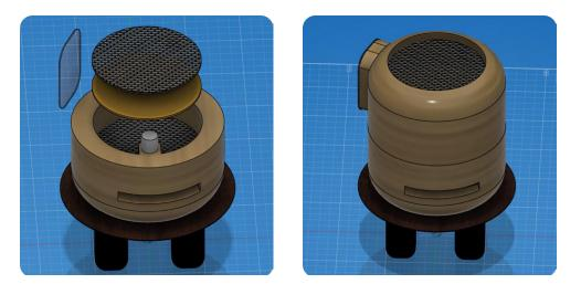
The prototype presents an intelligent hive divided into two sections: one for the bees' habitat and another for the automated and non-invasive extraction of apitoxin using electrostatic discharges.
