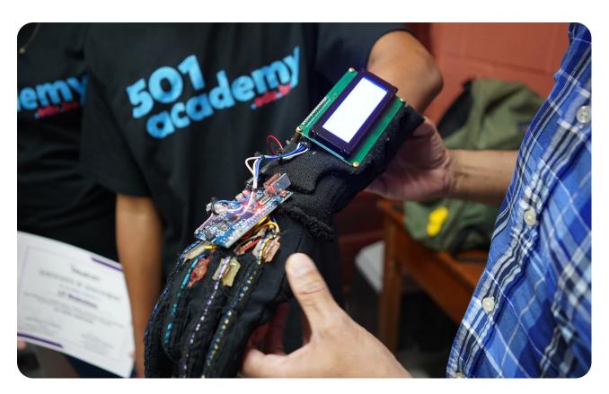
Powered by Arduino and flex sensors, this inclusive innovation translates finger movements into words displayed on an LCD screen—bringing low-cost assistive tech to life.
